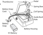
battery from the battery housing,
